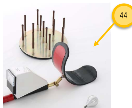
Figure 16 HV Head Component Attachments
